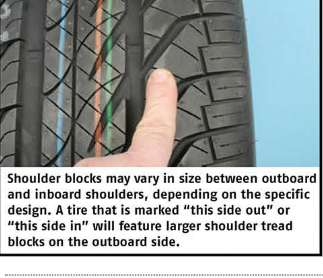
Angled grooves, referred to as lateral grooves, direct water out from the longitudinal grooves to aid in water evacuation. Water is collected in the main grooves and directed out of the tread area via lateral grooves.
