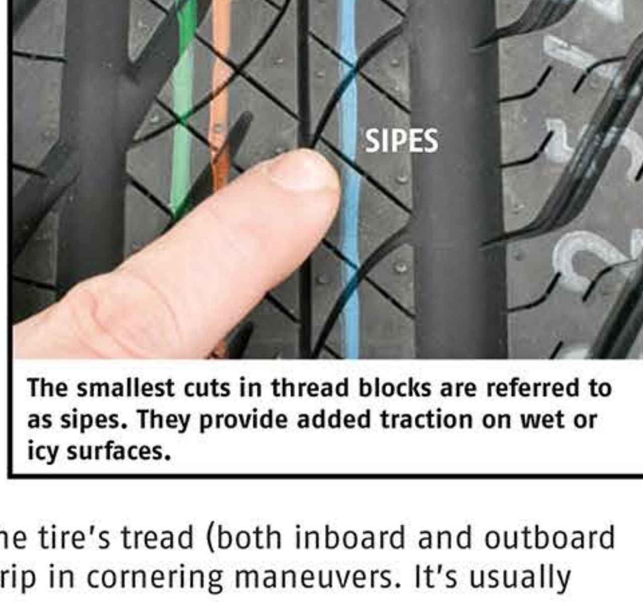
Longitudinal grooves in the tread allow for immediate water passage.
