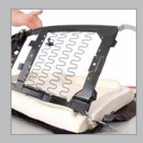
Placing the C4 Seat Bracket
